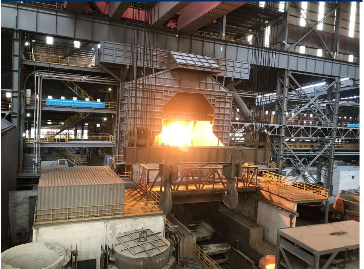
Figure 8: Argon Oxygen Decarburization Process at the IMIP
